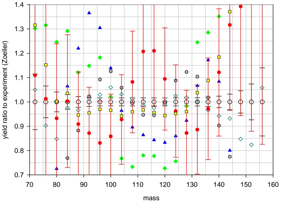
*Benchmark A:  $^{238}\text{U}$  at 100 MeV, post neutron emission yield ratio to experiment (Zoeller)
